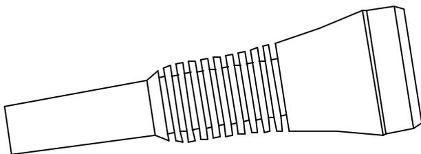
This model was developed in order to make extremely stable "slotting" possible. The "ribs" substantially enlarge the surface, leading to a larger vibrant surface. This form is only available by special order.
