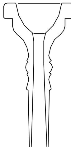
**2nd type** The cup is sectioned to the bore, in combination with a very flat rim, but has rounded edges.
