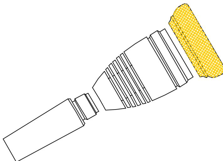
system is constructed so that the bore of the cup does not influence the bore of the shank. This design is an absolutely new product development. The “vibrating ribs” feature work extremely well with a “heavy” model, but with a slight reduction of mass. One has the feeling of setting on railroad tracks, but enough flexibility remains to make differences in tonal shading.
