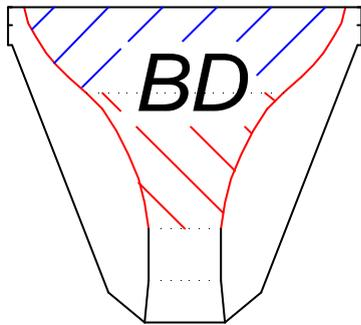
The **cup** determines the volume of tone, with forms varying from a *C-form* to a *V-form*.
