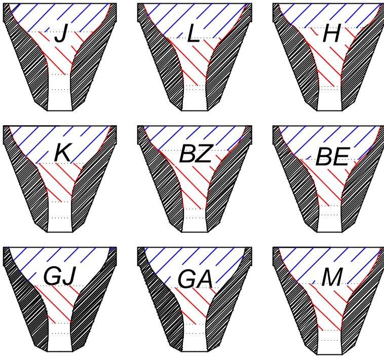
The symphonic cups of the larger category can be recognized by the 3 mm fitting. These are appropriate for a large, orchestral sound. In general, instruments with Perinet valves should have cups with a bowl-shaped form, while V-formed cups are more suitable for instruments with rotary valves.
