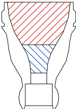
The **cup** determines the volume of tone, with forms varying from a conical form (V-form) to a bowl-shaped form. The throat (or junction to the bore) strongly influences the tone color, with a wide throat producing a darker tone, and vice versa.
