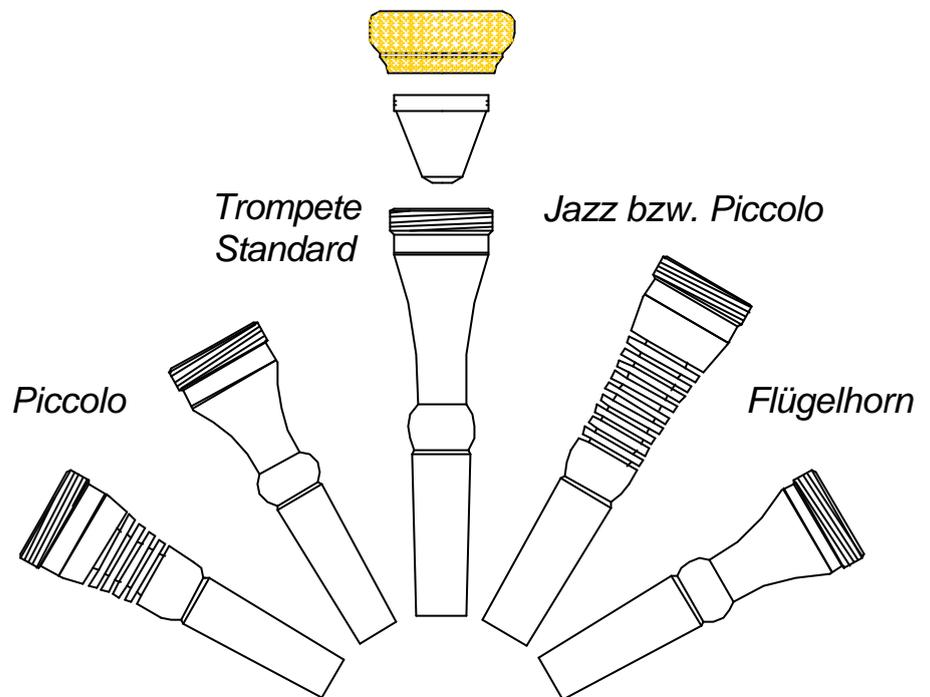
The cup diameter is measured at a depth of 2mm. The size standardization of the cup diameter (or internal rim) runs from the numbers 1 to 9, and the corresponding trumpet mouthpiece diameters range from 15.4 to 17.0 mm. The progression follows in increments of 0.2 mm.
