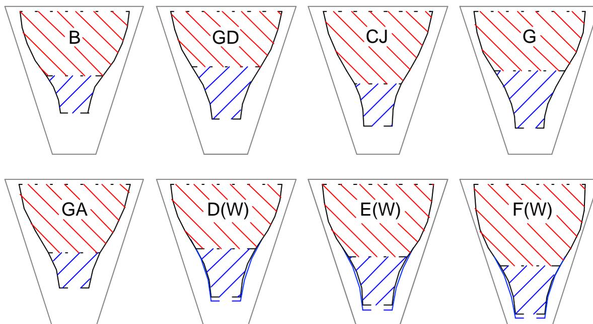
Addendum to cups *D – F*: a cup labeled “EW” is, in principle, identical to cup “E”. The only difference being that the “EW” has an extended throat (blue line) for providing a better air flow.
