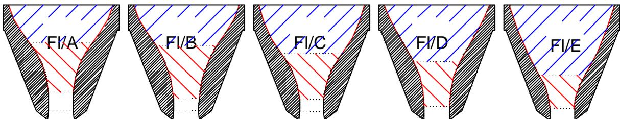
The flugelhorn cups are either combined with special, short shanks, or with trumpet shanks with the corresponding diameter. The small cups are very suited for playing in wind bands.
