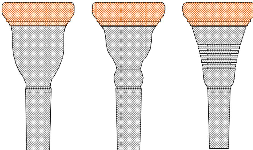
The model in the middle (\*) is the standard. The desire for light or heavy models should be indicated when ordering.
