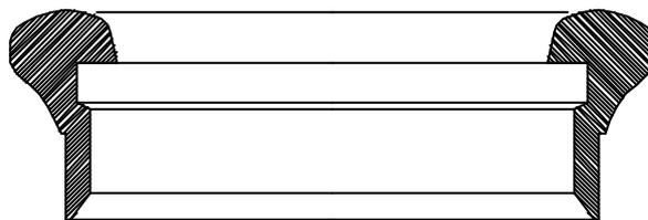
For a better overview, the overall descriptive character and the rim contour are, respectively, divided into four subsections: the inner edge or *rim bite*, *rim thickness*, the *outer rim edge*, and the *rim width*.
